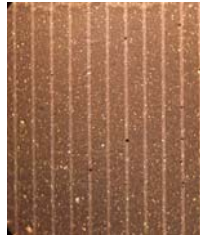
Optical micrographs of laser sintered tracks at 100 and 250 micron line spacing on paper
