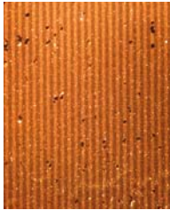
Optical micrographs of laser sintered tracks at 100 and 250 micron line spacing on paper
